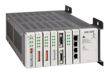
The Adit<sup>®</sup> 600 integrates VoIP gateway, IP access router, IP VPN, Firewall, channel bank, 1/0 DCS, CSU/DSU, and DLC in a compact chassis. The chassis is compact enough for two Adit 600s to be mounted side-by-side in a 2RU rack space. The high density architecture of the Adit 600 supports configurations up to 48 FXS or FXO ports, 18 T1s, or 12 10/100 interfaces.
